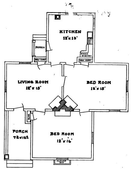
Fig. 32.—PLAN OF BETTER-TYPE COTTAGE SHOWN IN FIG. 31.
